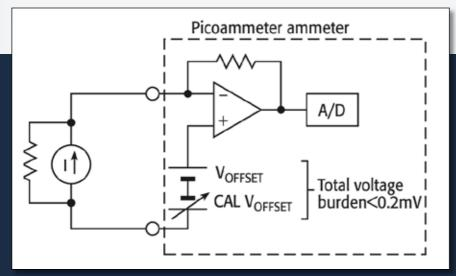
Unlike DMMs, picoammeters like the Model 6485 and 6487 employ a feedback ammeter design that reduces voltage burden dramatically for better measurement accuracy.
