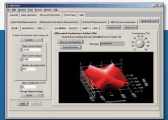
The 622X/2182A combination makes it simple to perform, analyze, and display differential conductance measurements.
