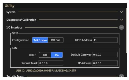
Figure 3: Set the GPIB address
